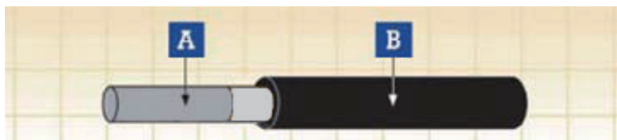
A. Conductor B. Insulation
